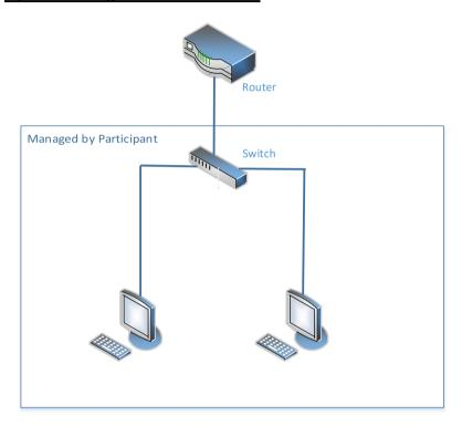
Option 2: Single Link Connection with Direct Connection to Router
