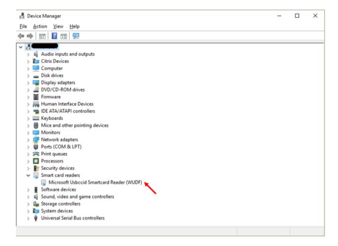
4. Double click on Microsoft Usbccid Smartcard Reader (WUDF). Ensure Device status is "This device is working properly".
